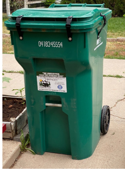
Strap Design-retrofitted trash can. Photo credit: Daniela Kohl
